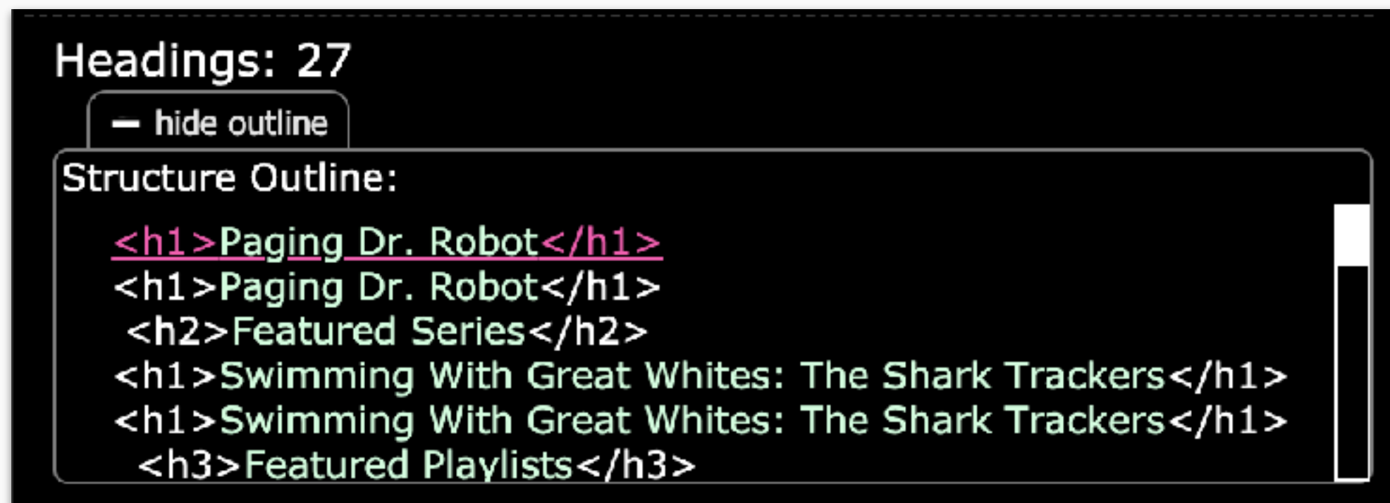
Screenshot, ANDI Audit. Heading structure, many duplicates and skipped heading levels (H1 → H3)
